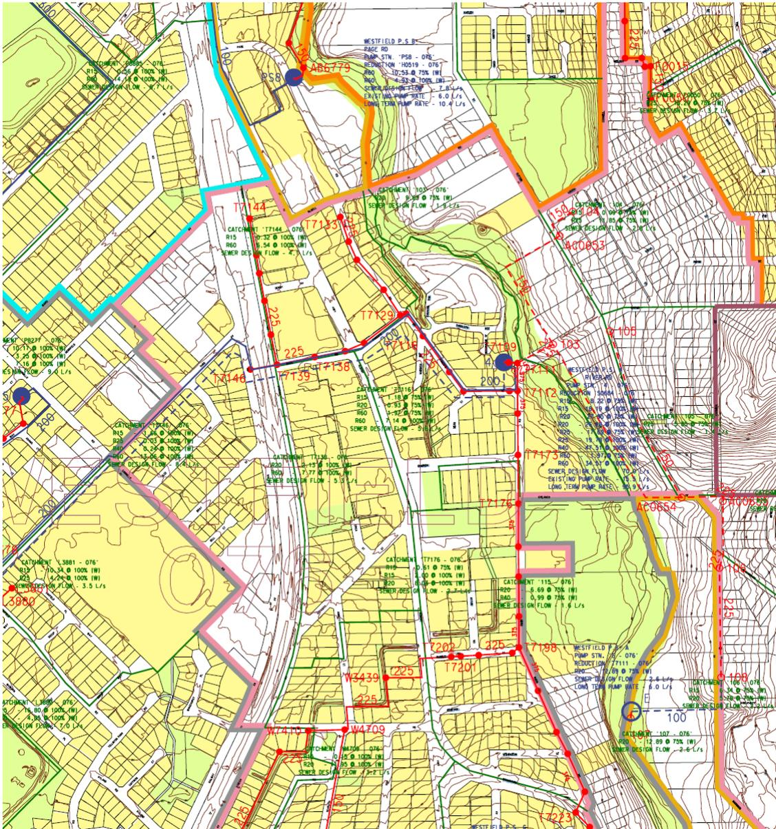
The gravity sewers are shown in red and the pump stations as blue circles.
