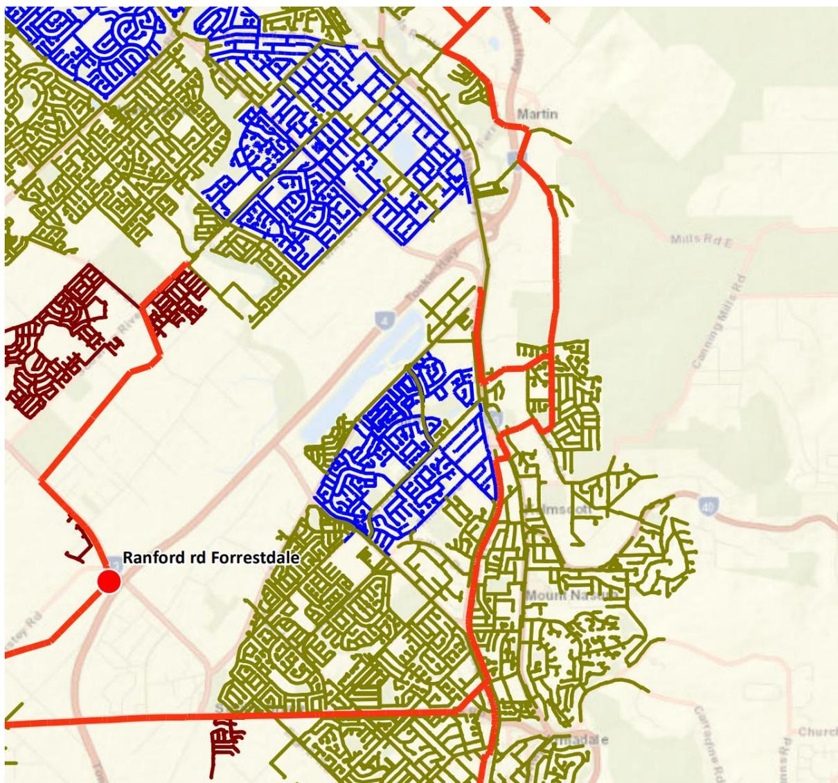
*Medium pressure gas mains are shown in orange. Medium-low pressure gas mains are shown in blue.*
