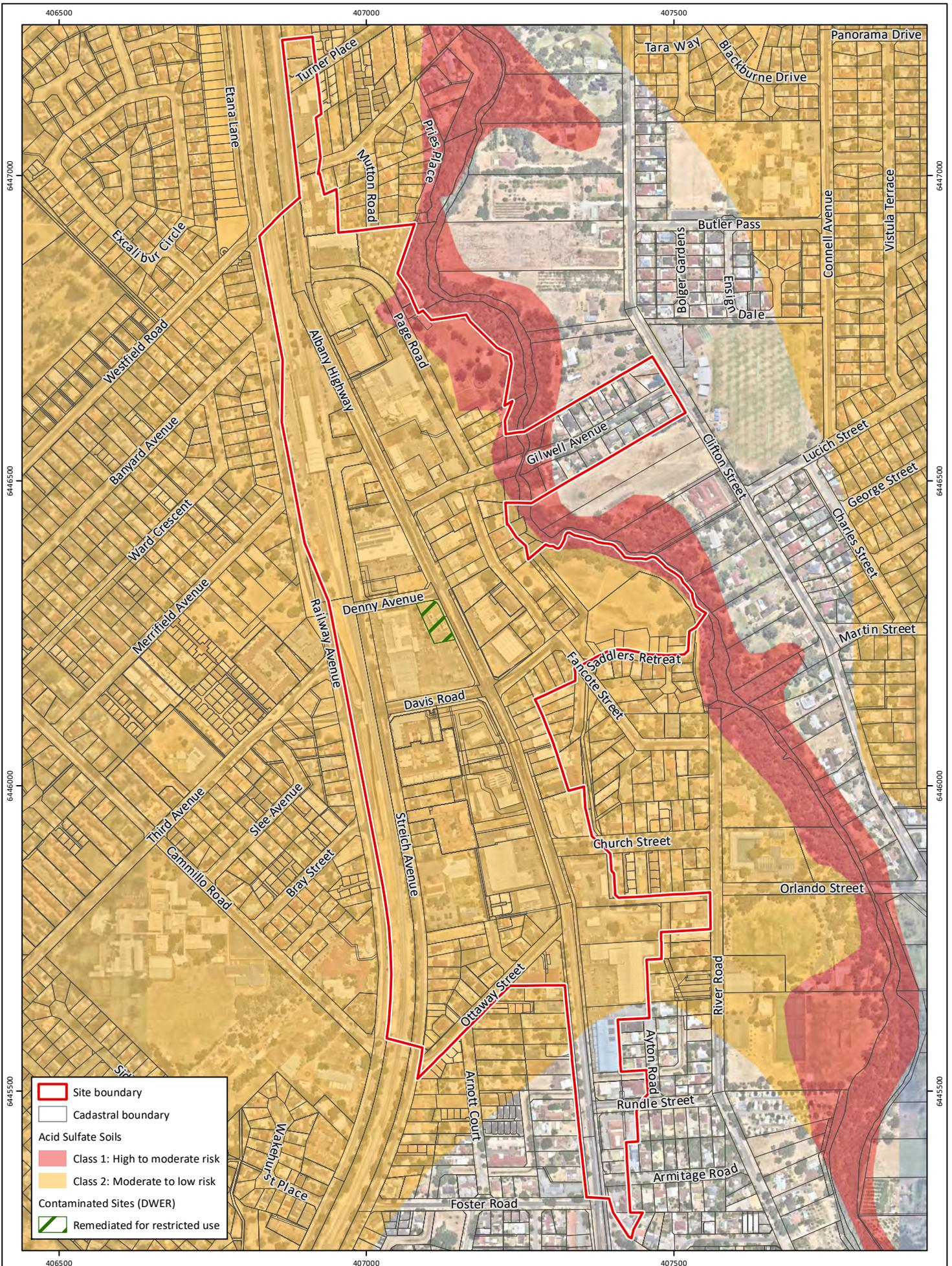
**Figure 4: Acid Sulfate Soils and Contaminated Sites**
