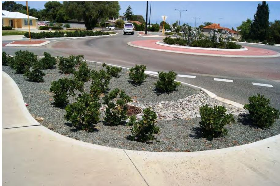
Plate 2: Example of bio-retention area in road verge
