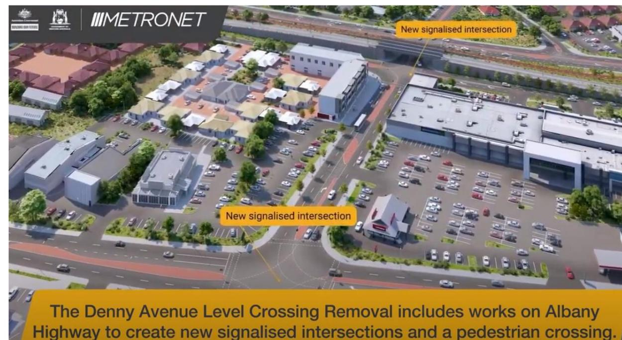
Figure 44 New signalised intersections at Albany Highway and Davis Road and either side of the new Davis Road underpass
